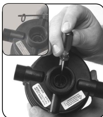
Trin 5. Afmontér #17 O-RING.
