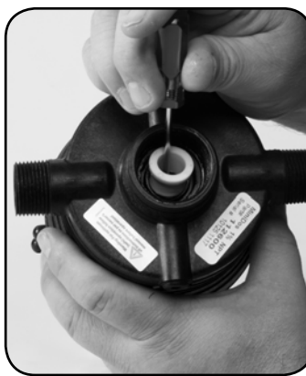
Step 5. Replace #83 SHAFT SEAL SPACER.
