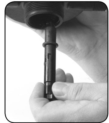
Step 6. Re-install #52 UPPER SHAFT and #17 O-ring.
