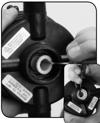
Step 7. Replace #82 SHAFT SEAL SPACER and #16 Gasket.
