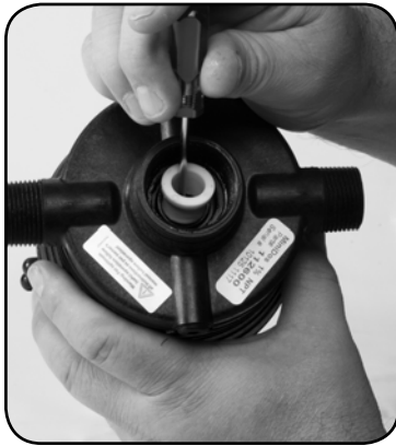
Step 4. Remove #82 SHAFT SEAL SPACER.
