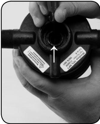
Step 4. Remove #17 O-ring and replace.
