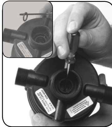
Schritt 5. Remove #17 O-ring.
