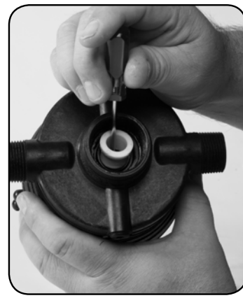
Step 3. Remove #83 SHAFT SEAL SPACER.
