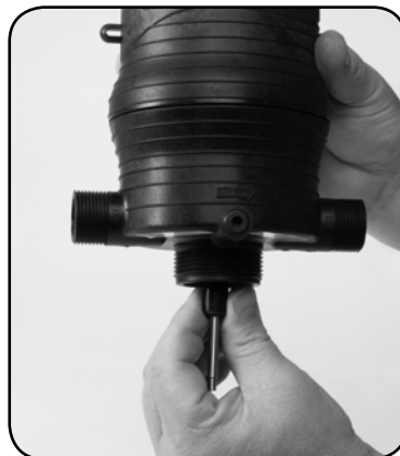
Step 8. Replace #51 SHAFT ASSEMBLY.
