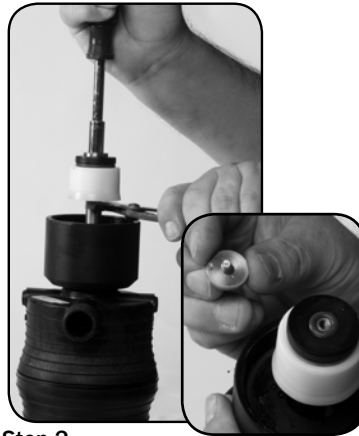
Step 2. Unscrew to unlock and remove #93 CAPSCREW.
