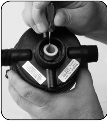
Schritt 4. Remove #82 SHAFT SEAL SPACER.
