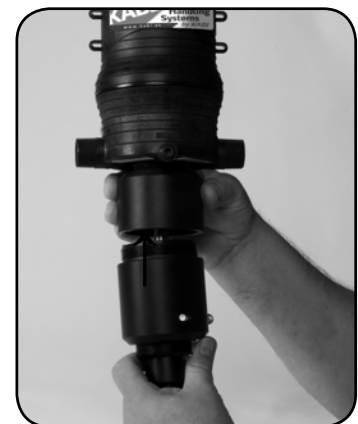
Step 9. Screw #61 OUTER CYLINDER onto body.
