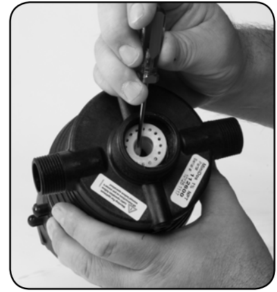
Step 3. Remove #16 Gasket.
