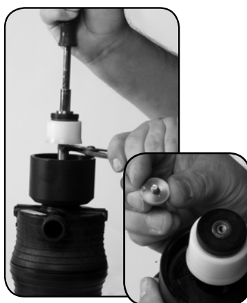
Trin 2. Skrue for at afmontere #93 CYLINDERSKRUE.
